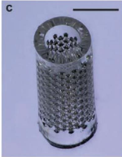
Micro filter element with 55 um holes
